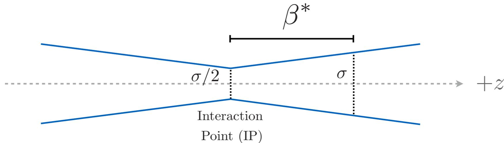
Normally, low optics  $\rightarrow$  small beams  $\rightarrow$  large luminosity
